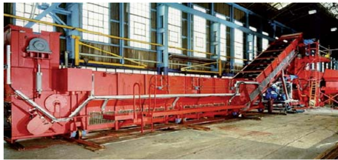
Figure 7: SSC Factory Assembled for Testing
